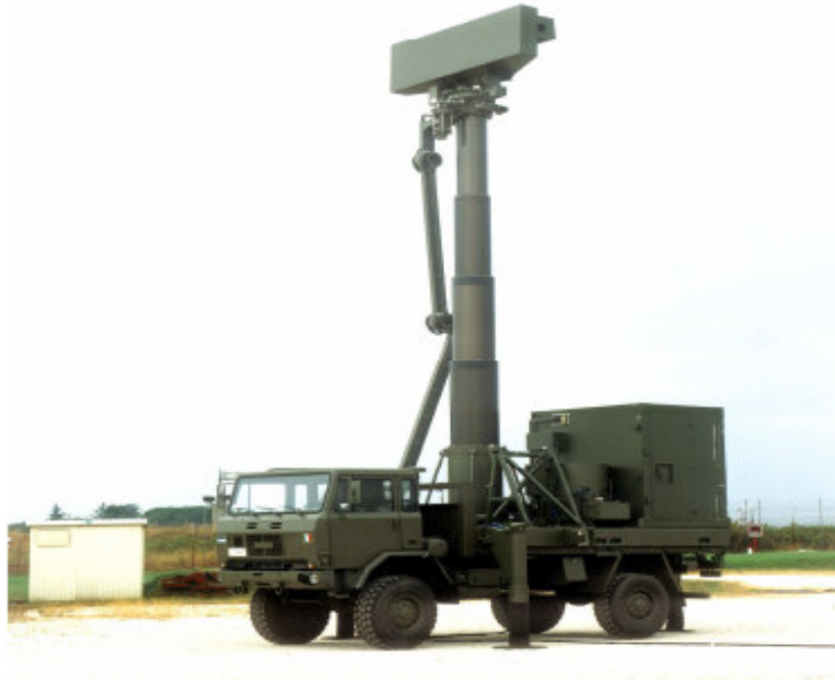
Figure 10: SELEX ARGOS-45 C-band radar in road transportable configuration (image courtesy of SELEX-SI Ltd).
