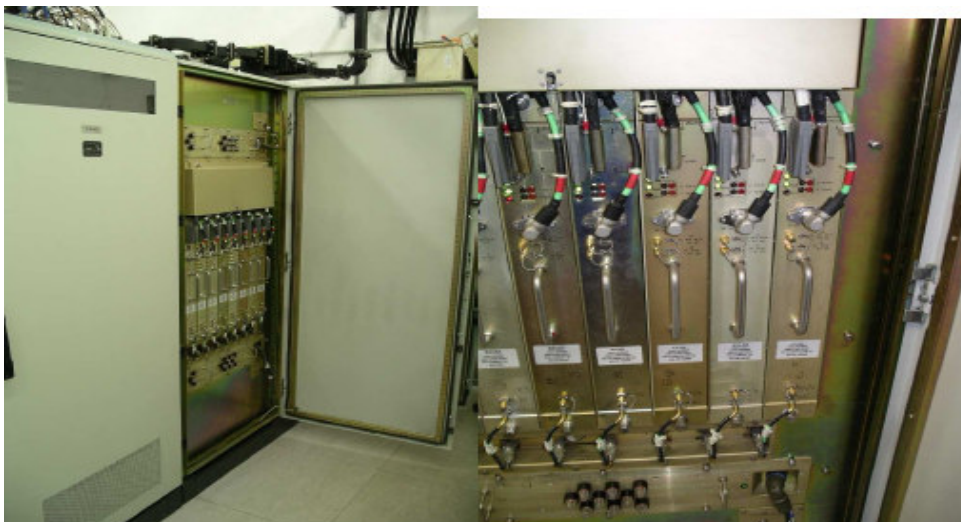
Figure 9: SELEX S-Band solid state transmitter for conventional and phased array antennas. (Images courtesy of SELEX-SI Ltd).
