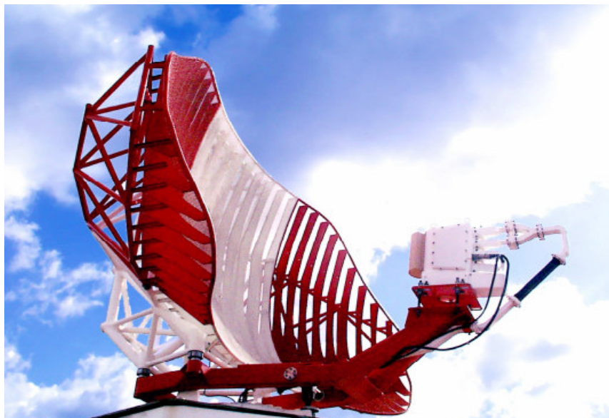
Figure 7: Conventional antenna for SELEX APCR-33S radar (image courtesy of SELEX-SI Ltd).
