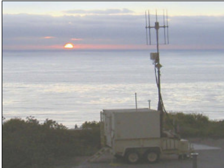
Figure 13: Lockheed Martin SILENT SENTRY passive coherent location sensor (image courtesy of Lockheed Martin).
