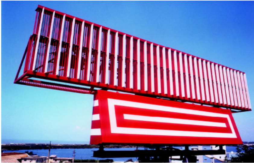
Figure 8: SELEX SI ATCR-33S radar with phased array antenna. (Upper antenna is for an associated secondary surveillance radar.). Image courtesy of SELEX-SI Ltd.
